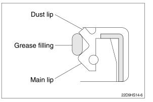
(9) Fill the oil seal into the hole by using the oil seal guide and oil seal snap.
